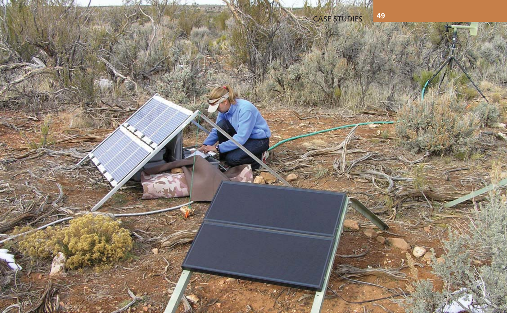
Figure 2. Laura Levy checks the acoustic monitoring station for the Fossil Canyon general aviation corridor at Grand Canyon National Park. The solar arrays measure approximately 24 x 30 inches and 42 x 30 inches.
