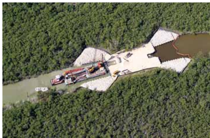
Figure 3. Aerial view of nearly completed dam at East Cape Canal, Cape Sable, Everglades National Park. The dams are expected to add resilience to upstream freshwater ecosystems by reducing unnatural intrusion of saltwater into the area.
