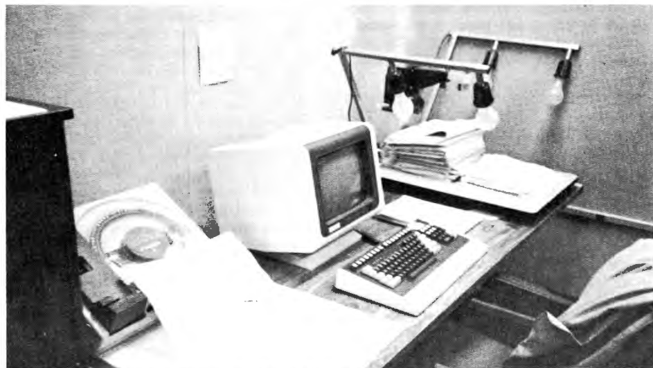
Two offices, similar to this, were created from a single vehicle bay. Acoustical wall paneling and carpeting on the floor minimize sounds. A keyboard and video display in each office is hard-wired to the computer operating system in the administrative area.
