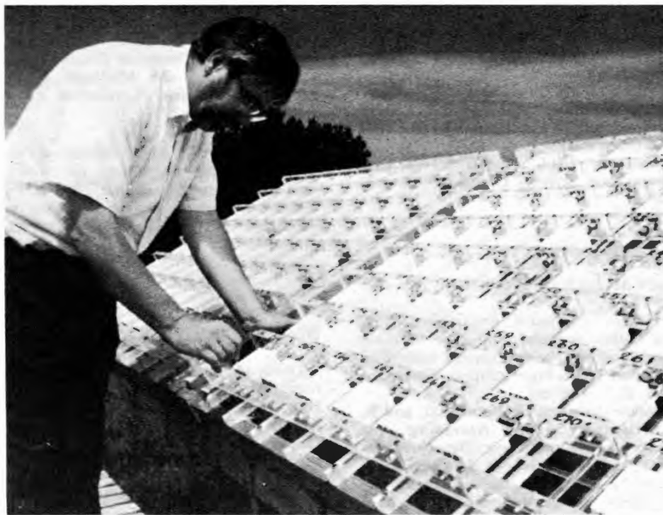
A technician examines a field exposure test rack with Vermont marble (foreground) and Indiana limestone (background) at Research Triangle Park, NC.
