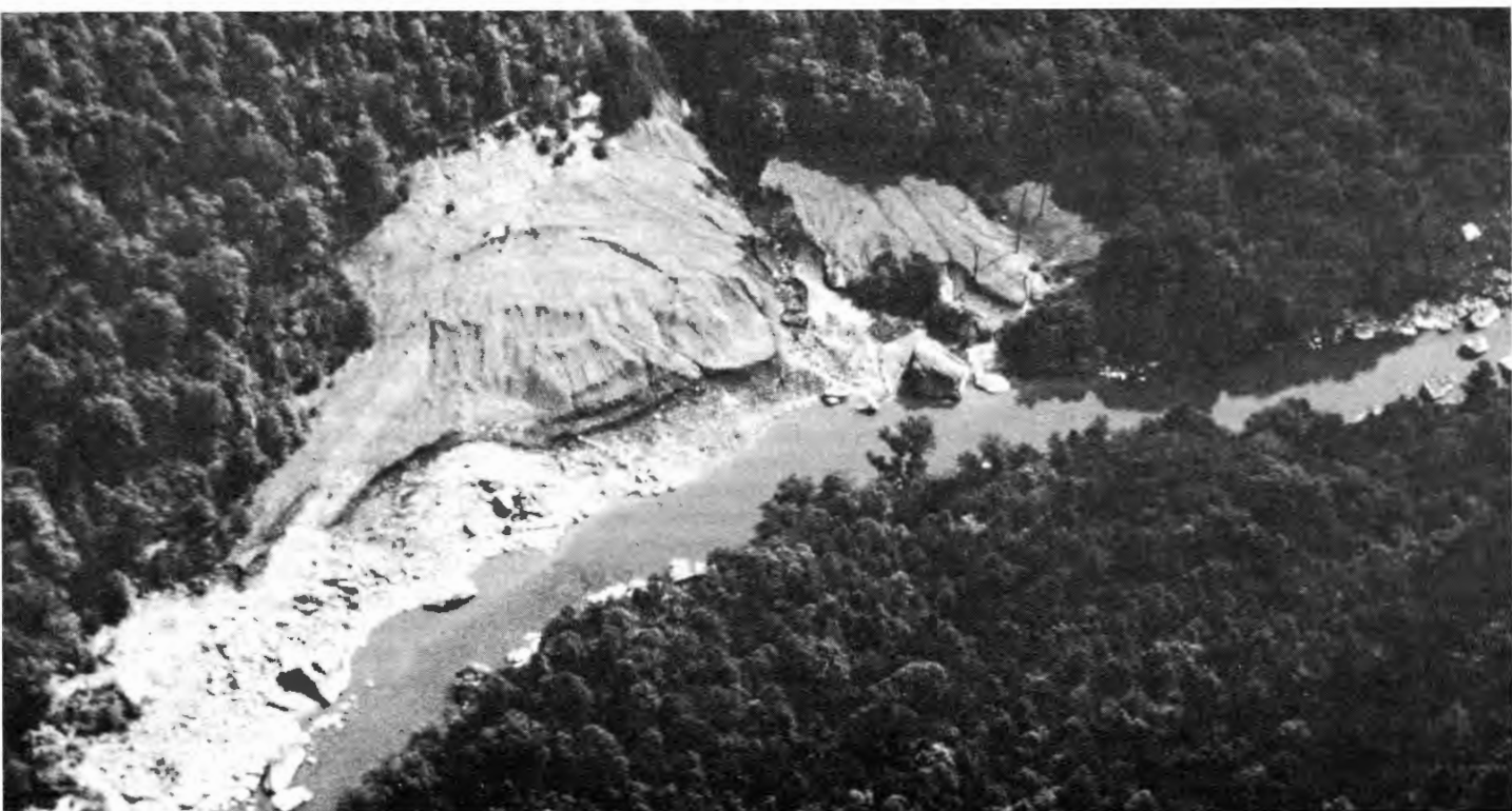
Mine spoil embankments along the Big South Fork of the Cumberland River, Big South Fork NRRRA. The highly acidic, pyritic shale in these spoils prevents natural revegetation and adds to erosion and acid runoff problems.
