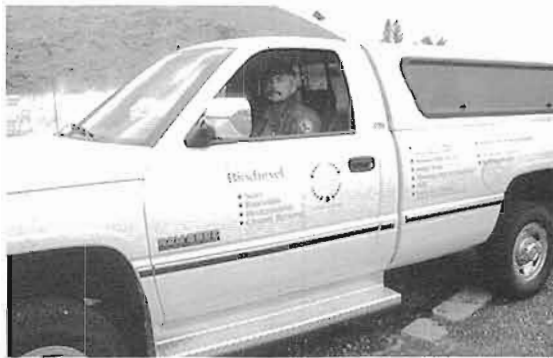
Fueled by biodiesel or rapeseed (canola) ethyl ester, this pickup truck has traveled more than 115,000 miles in and around Yellowstone since 1995, averaging 17 miles per gallon. Engine and fuel system modifications were not needed, and emissions of smoke, hydrocarbons, nitrogen oxide, and carbon monoxide were reduced compared to regular diesel.
