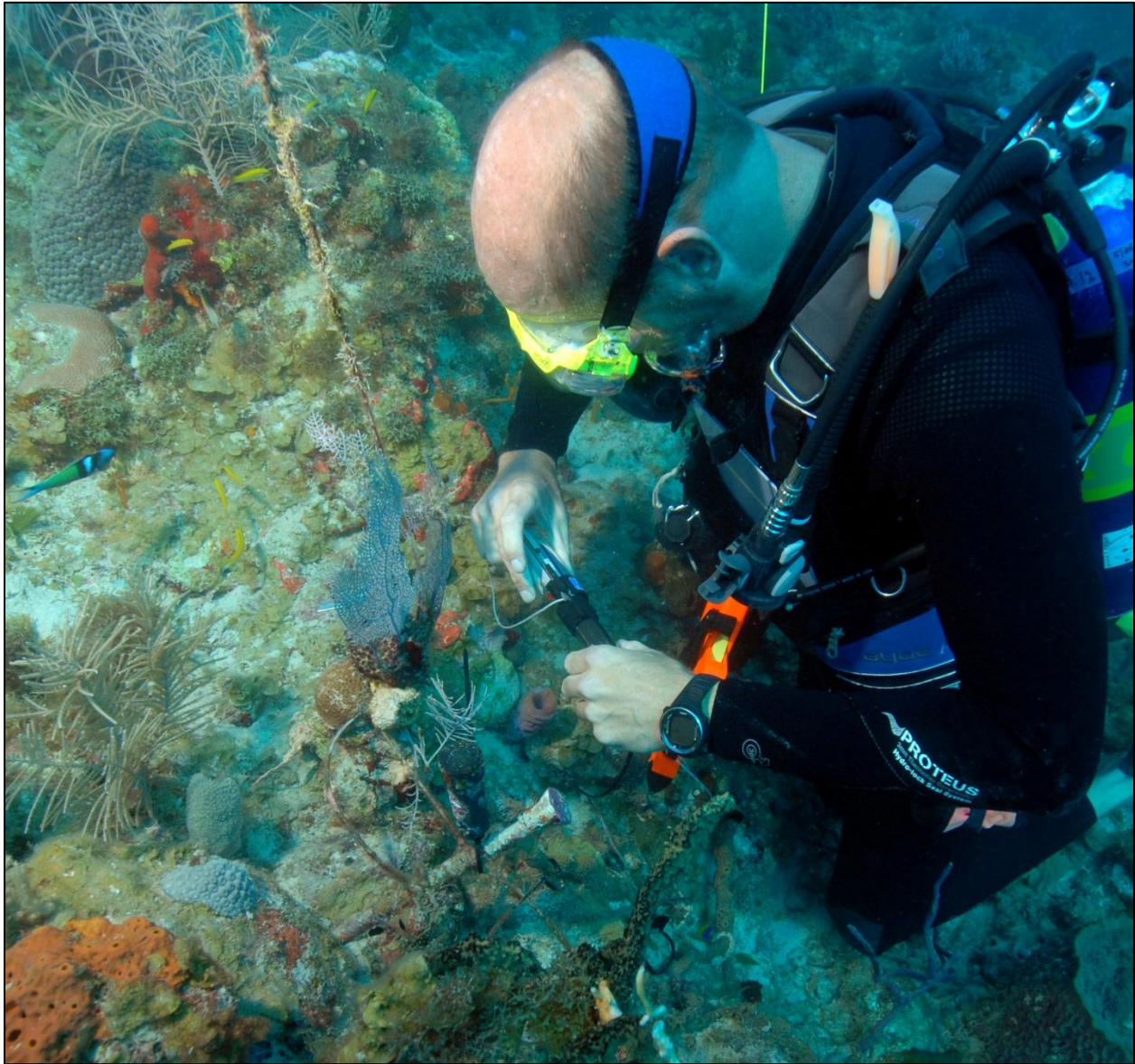
Brian Witcher downloads reef temperature data with a HOBO ® waterproof data shuttle in DRT0 (Photo credit: Rob Waara).
