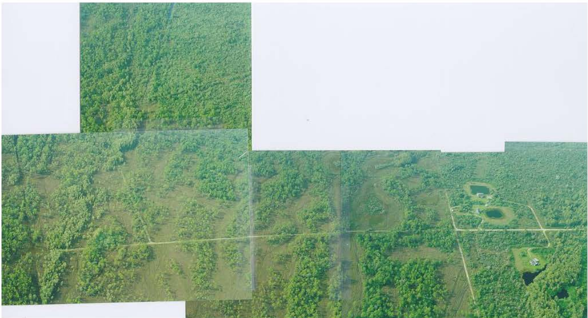
Photograph 2. Aerial view of non-residential east end of Bass Lake Estates, looking south. All elevated roads to the left of the borrow pits will be removed under this project.
