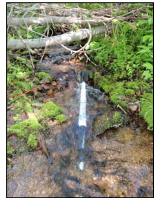
Little Cottonwood Creek (CRMO), continuous water quality monitor
