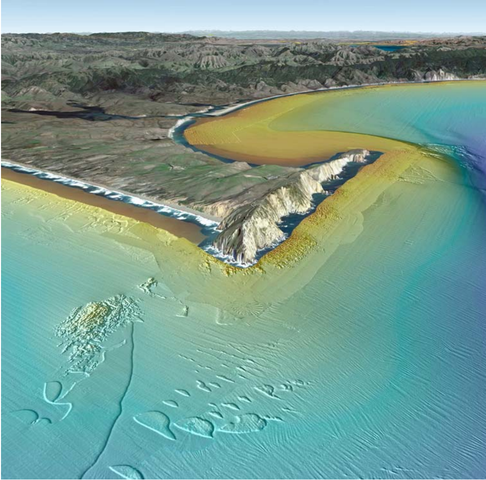
Figure 5. A MBES bathymetric image showing dynamic bedforms of mobile sand sheets and dunes being swept by bottom currents around Point Reyes Headlands. Note bedrock outcrop on seafloor that is an extension of the headland. Striations on seafloor are artifacts from the roll of the survey vessel.
