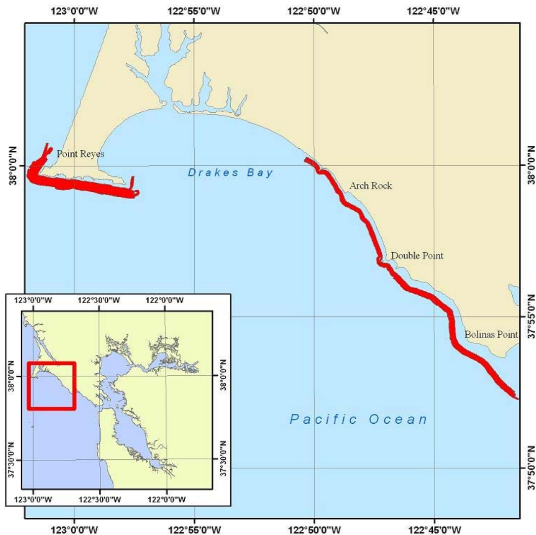
Figure 2. Area of coverage of interferometric side-scan sonar data collected with a GeoSwath 240 kHz bathymetric mapping system used by MLML Center for Habitat Studies initial marine benthic habitat characterization study (Modified after Erdey-Herdorn, 2007).
