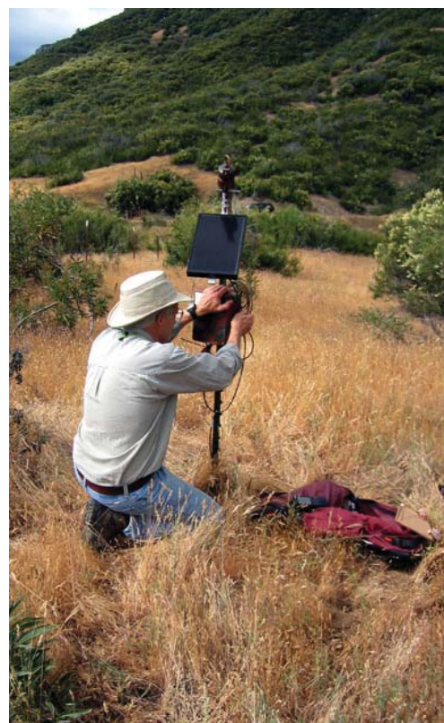
Bill Rainey setting up a bat detector to record bat calls in the Shepherd Saddle area. A solar panel charges the battery that powers the AnaBat detector, and bat calls are stored on a small memory card. Photo: Elizabeth Pierson.
