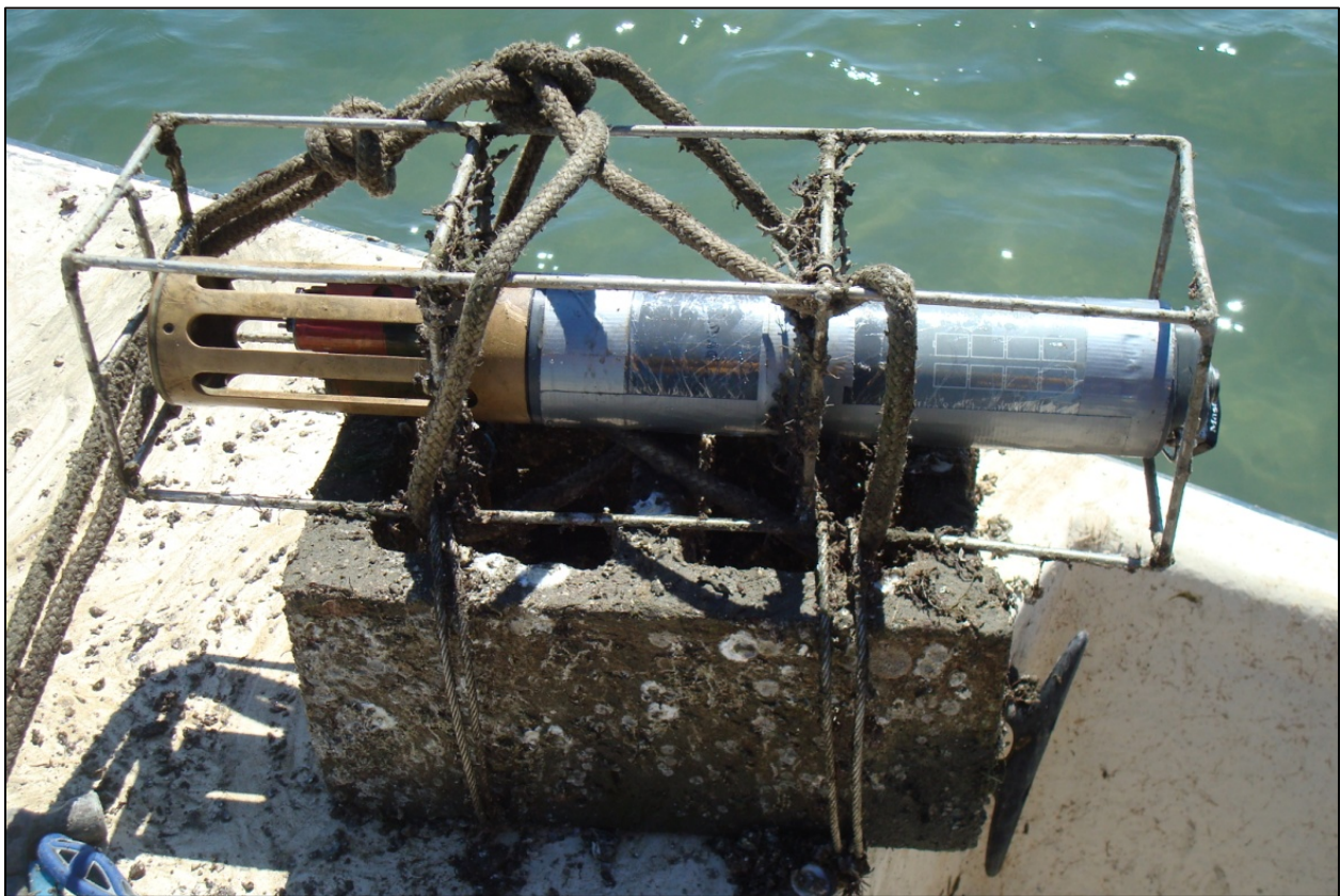
Figure 2. Photo of continuous data collection sonde mount used at Middle Marshes (CALOshak2) at Cape Lookout National Seashore. Photo by John Fear, NCNERR staff.
