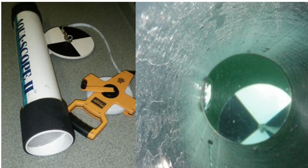
A Secchi disk helps measure a water body's transparency level. Pictured are a Secchi disk, measuring tape, and viewing scope (left) and view of submerged Secchi disk through viewing scope (right). NPS photos.
