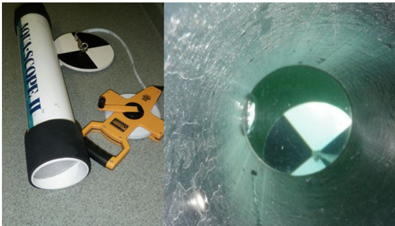
A Secchi disk helps measure a water body's transparency level. Pictured are a Secchi disk, measuring tape, and viewing scope (left) and view of submerged Secchi disk through viewing scope (right). NPS photos.
