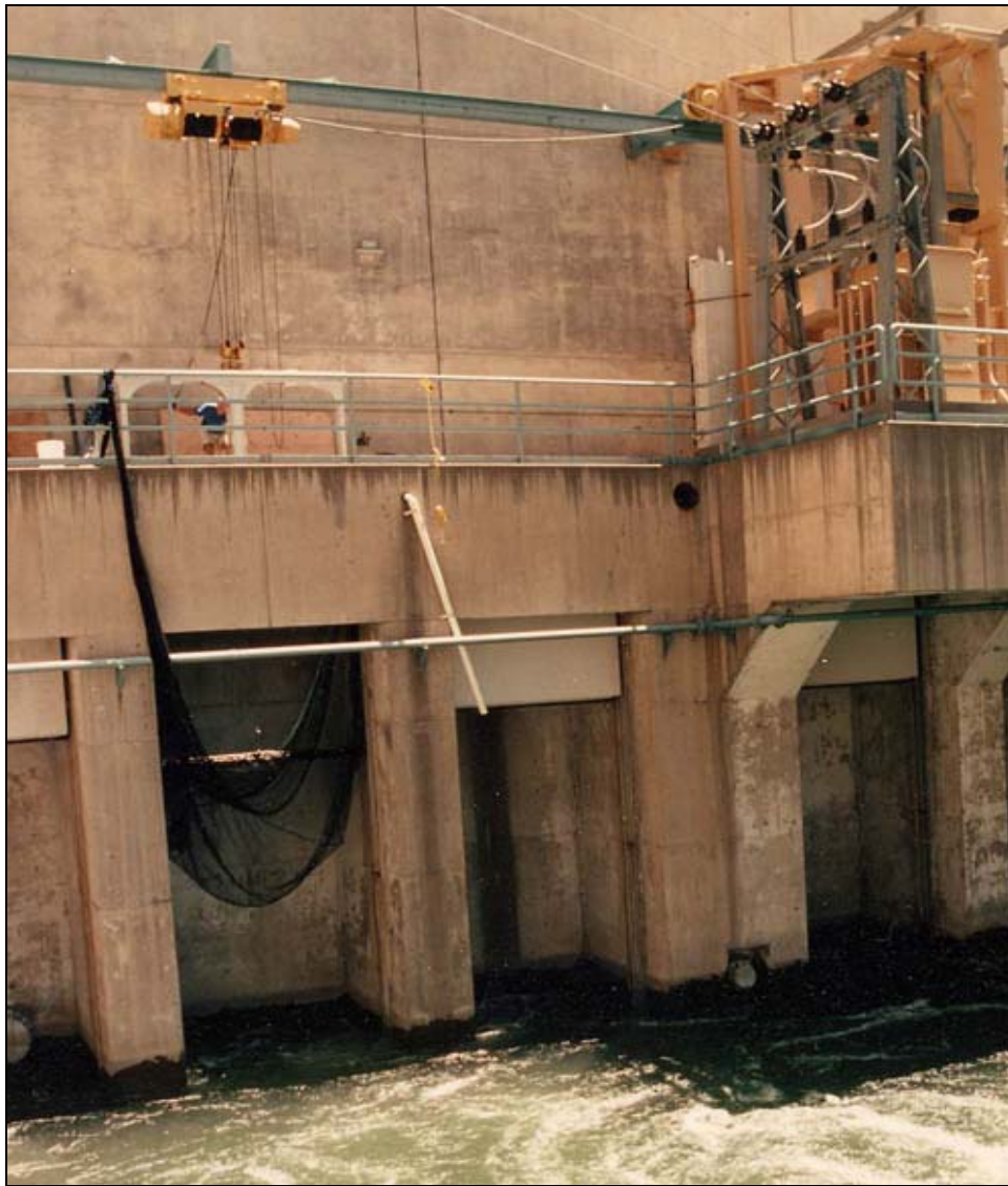
Figure 77. Sieve net used by Mueller and Hiebert (1997) to sample the outflow from one of the turbines below BMR dam.
