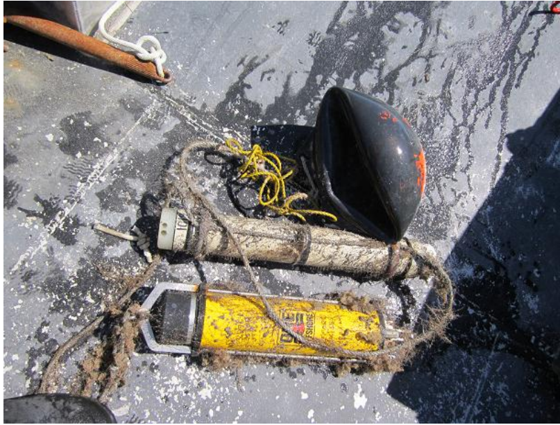
Figure 2: Grand Wash mooring recovered in June 2013. The black spherical subsurface float is collapsed and punctured.
