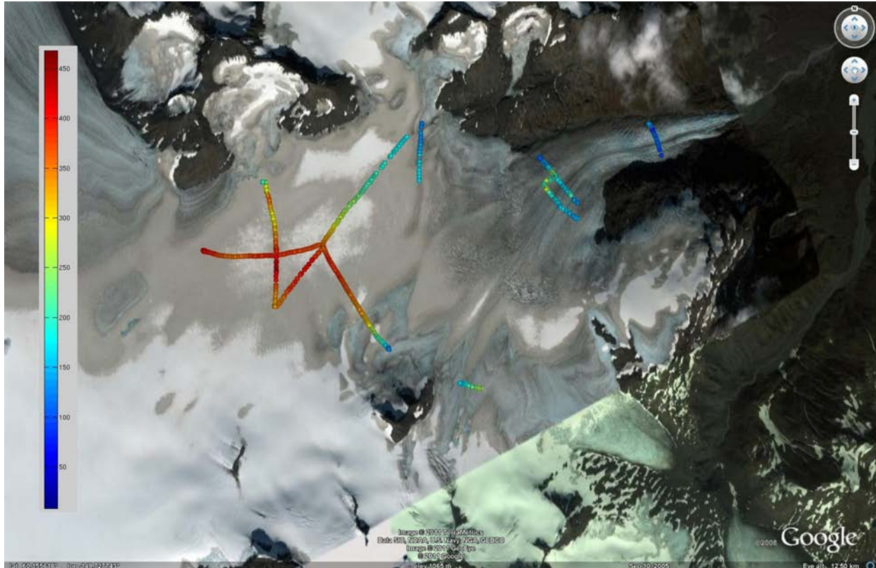
Figure 4. Ice depths derived from a ground-based radar survey of the upper Exit Glacier. The background image is from Google Earth. The transects are color coded with ice depth in meters.
