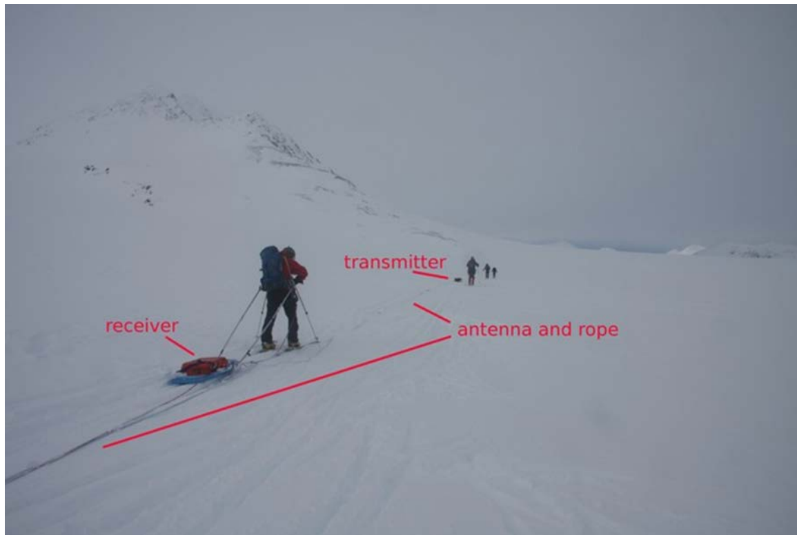
Figure 1. Ground-based radio echo sounding survey. The transmitter and receiver are towed on sleds that are separated by resistively loaded antennas.
