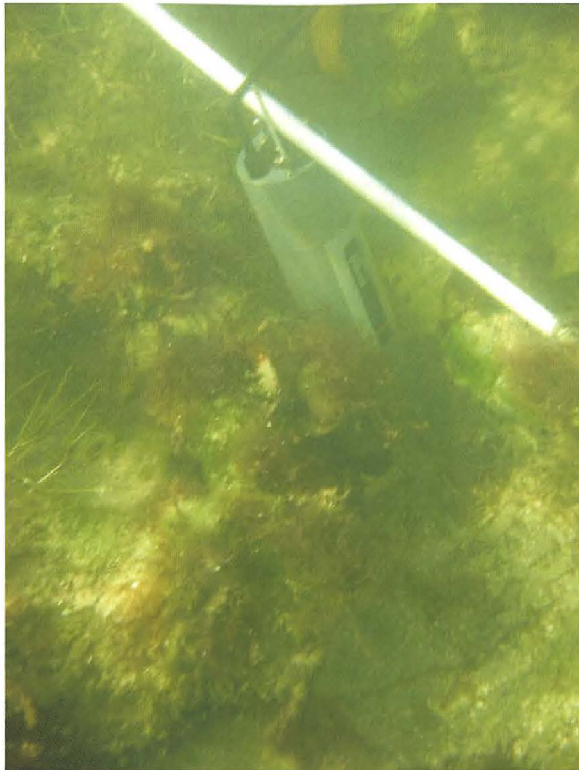
Figure 4: YSI instrument deployed within a conduit of BBS21
