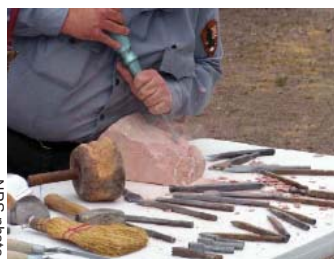
Shaping stone with the Dallet hammer and plain chisel (2009).
