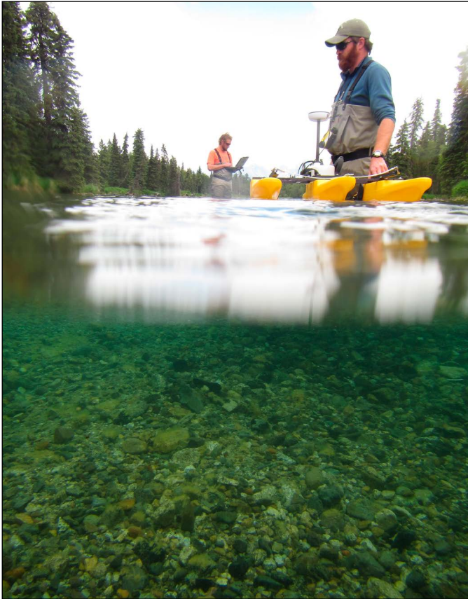
Biological technicians, Evan Booher and Jeff Nelson get set up to take a discharge reading on the little Kijik River (one of the most productive sockeye salmon streams in the park) in Lake Clark NPP with the Acoustic Doppler Current Profiler.
