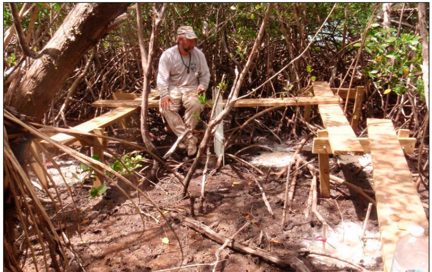
Figure 3 (right). SET sampling arm attached to newly installed benchmark, feldspar accretion plots (white powder material) are visible.
