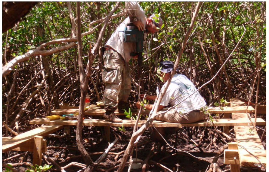
Figure 2. Jack-hammering survey rods into bed rock until geological refusal is obtained.
