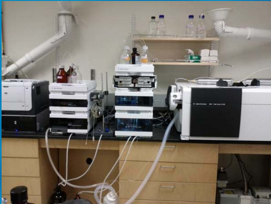
Compound detection (Agilent 6460 LC-MS/MS) Liquid chromatography combined with tandem mass spectroscopy
