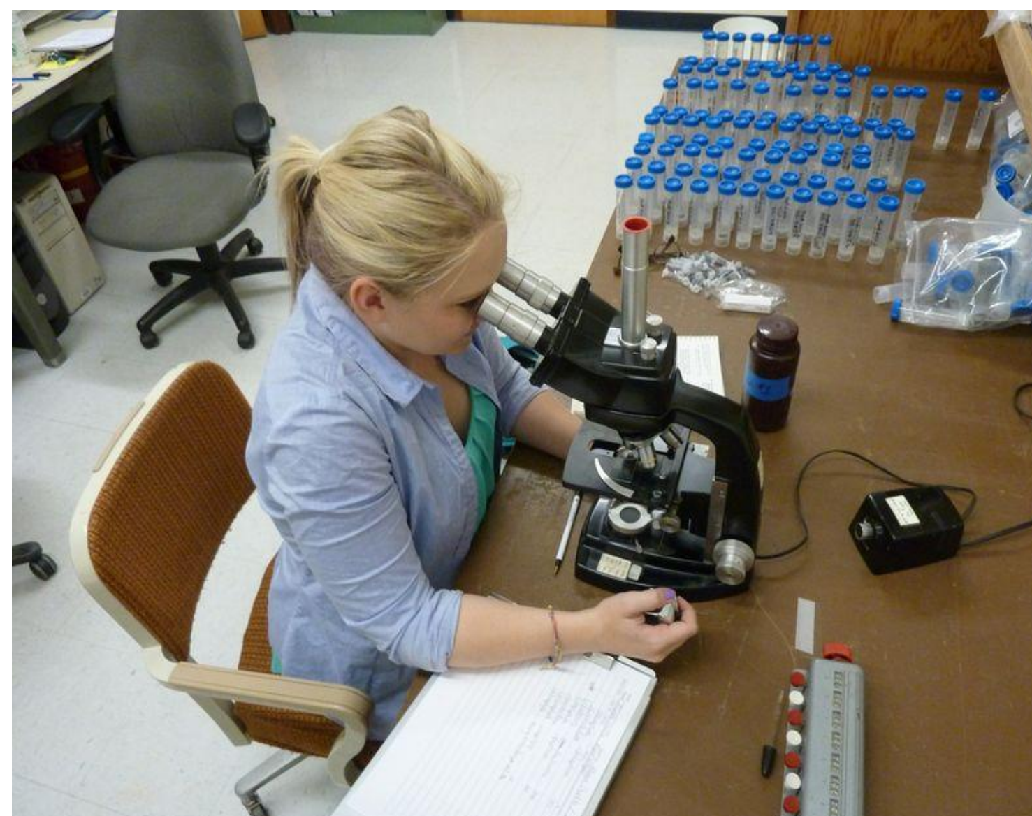
Figure 5: Microscope evaluation of algal samples using Sedgwick-Rafter slide to determine algae genus and biomass
