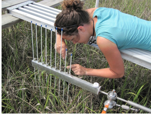
Figure 10. RSET with fiberglass pins being lowered to the marsh surface.
