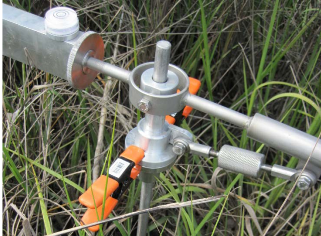
Figure 9. Clamp RSET to collar using spring clamps.
