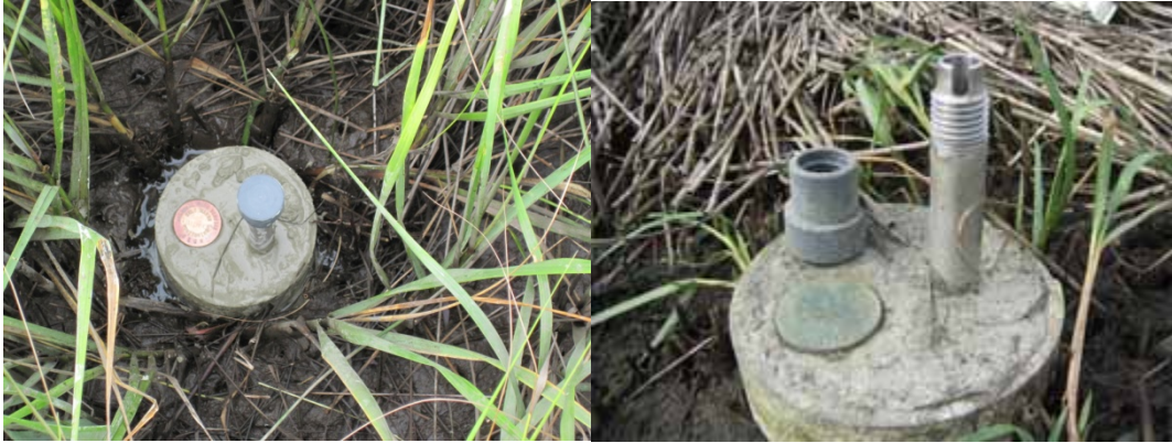
Figure 4. Deep rod benchmark / monument and receiver capped (left) and receiver uncapped (right from USGS Taking your SET readings page: http://www.pwrc.usgs.gov/ )
