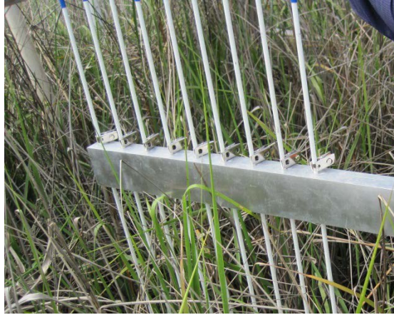
Figure 6. Fiberglass pins installed in RSET with badge clips.
