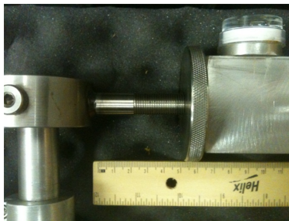
Figure 5. RSET arm locked into position 6 cm from the exterior edge of the pivot joint.
