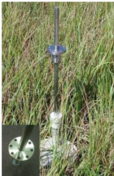
Figure 7. RSET insert collar mounted to receiver. Inset: insert collar close-up. (modified from USGS Taking your SET readings page: http://www.pwrc.usgs.gov/ )
