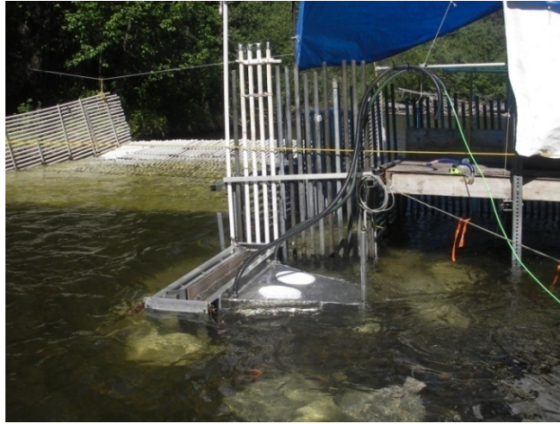
Figure 7. Underwater video and fish passage chute attached to weir.
