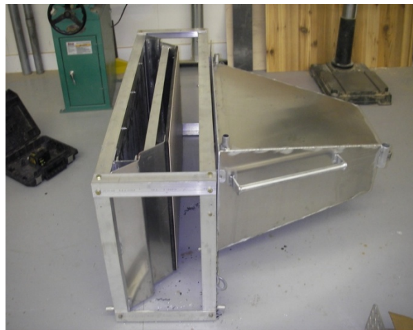
Figure 5. Video camera housing attached to fish passage chute.
