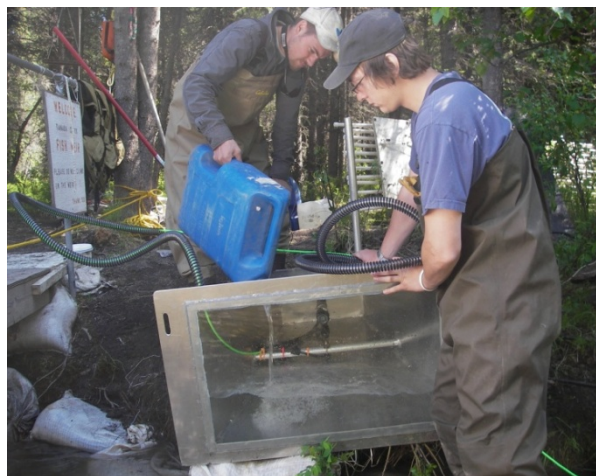
Figure 6. Preparing camera housing for placement in river.
