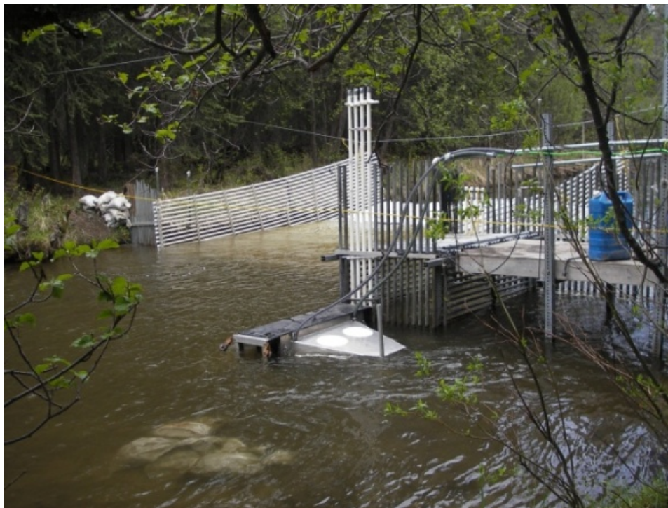
Figure 7. Underwater video and fish passage chute attached to weir, 2008.
