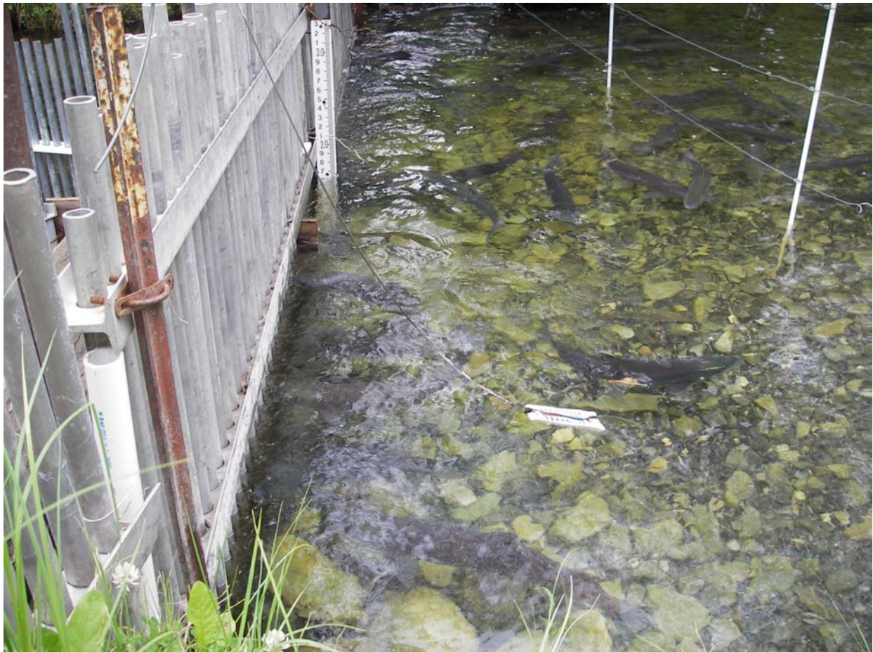
Figure 6. Staff gauge at Long Lake weir, 2006.
