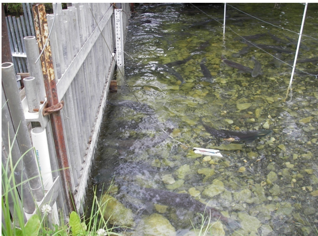
Figure 6. Staff gauge, electric bear fence, water surface thermometer at Long Lake weir, 2006.
