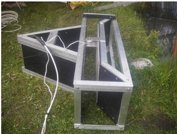
Figure 4. Camera box and fish passage chute.
