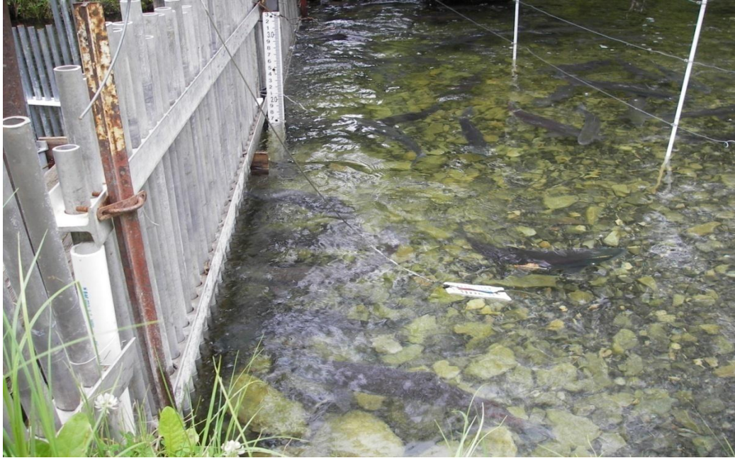
Figure 7. Staff gauge, electric bear fence, water surface thermometer at Long Lake weir, 2006.
