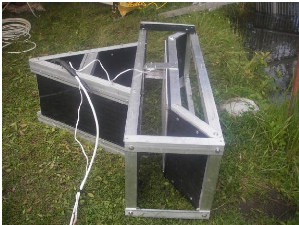
Figure 4. Camera box and fish passage chute.
