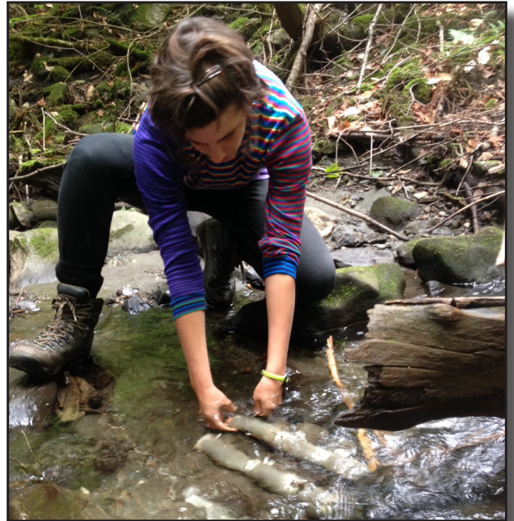
NETN Water quality monitoring intern Liza Mcelroy sets up continuous data loggers in Marsh-Billings-Rockefeller NHP's Pogue Brook. NPS photo.
