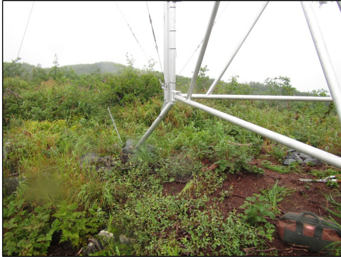
Figure 40. Pedersen Lagoon RAWS – Abundant vegetation grows around the weather station each summer. Plant growth is incidentally documented by the snow depth sensor which recorded a growth spurt beginning around June 9.
