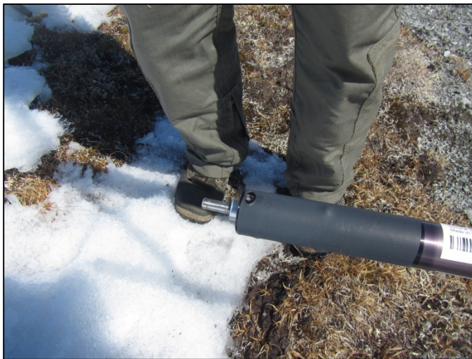
Figure 3. Chigmit Mountain RAWS – Wind vane missing from wind direction sensor.
