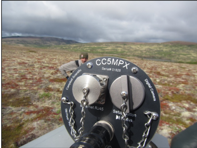
Figure 13. Coville RAWS phenocam – The Campbell Scientific time lapse camera was replaced with this updated version of the same equipment.
