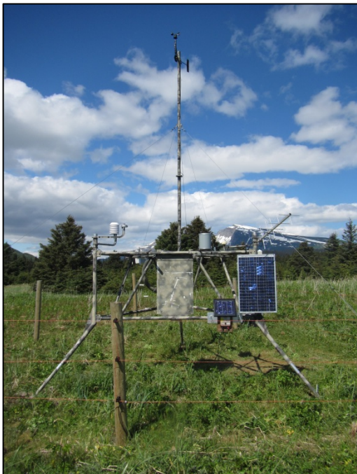
Figure 52. Silver Salmon Lakes RAWS – Station viewed from south after maintenance.
