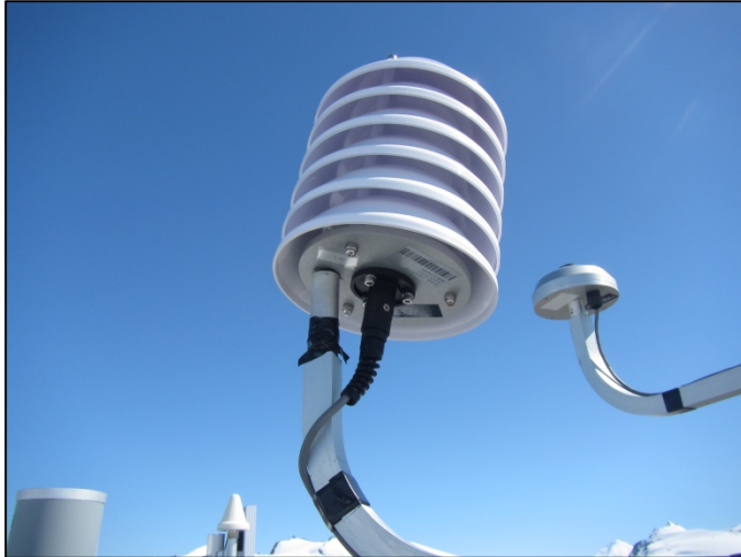
Figure 4. Chigmit Mountain RAWS – Loose mount on AT-RH sensor.
