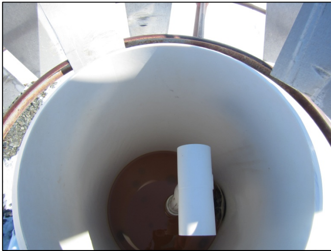
Figure 26. Harding Icefield RAWS – View down precipitation gauge. No ice was present.
