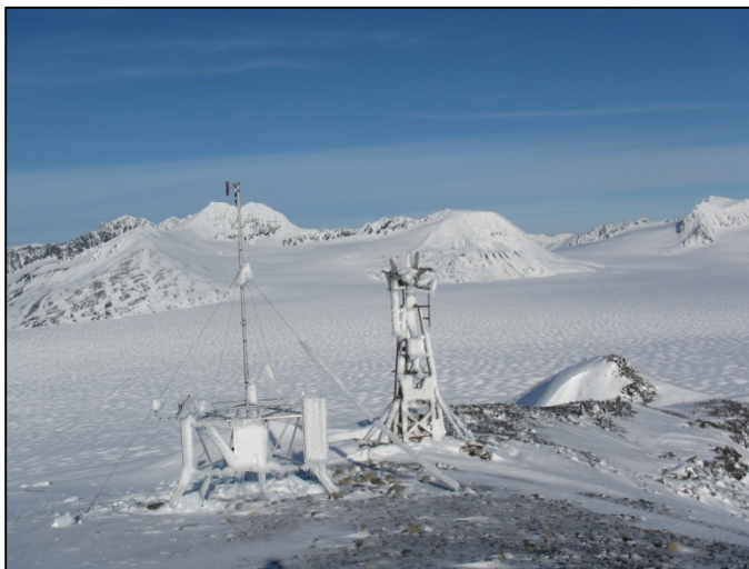
Figure 20. Harding Icefield RAWS – Rime ice covers the weather station.
