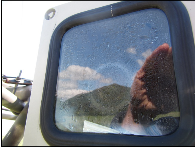
Figure 55. Silver Salmon Lakes phenocam – Moisture inside the phenocam housing.
