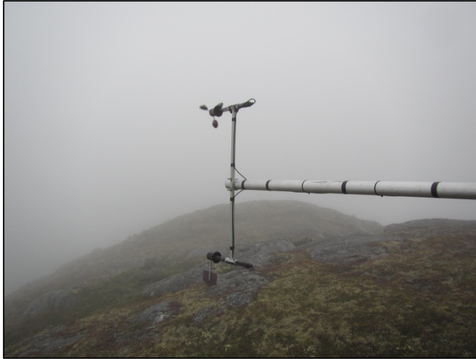
Figure 37. McArthur Pass RAWS – The fletching (tail) had fallen off the wind direction sensor.
