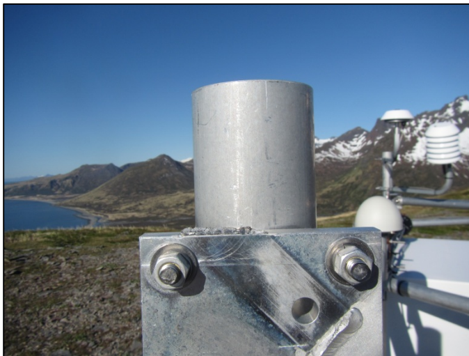
Figure 16. Fourpeaked RAWS – The GOES antenna mount broke.
