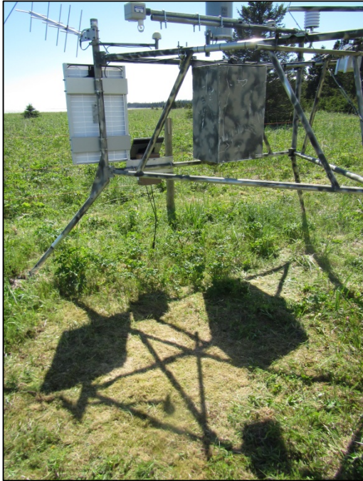
Figure 51. Silver Salmon Lakes RAWS – Judd snow depth sensor and snow depth target cleared of vegetation.
