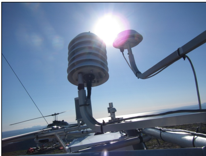
Figure 17. Fourpeaked RAWS – Loose mount on AT-RH sensor.
