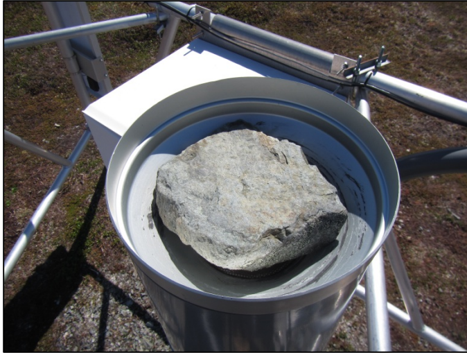
Figure 45. Pfaff Mine RAWS – A large rock was placed inside the tipping bucket in order to mitigate excessive tipping that occurs during strong wind events.
