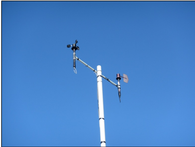
Figure 29. Harding Icefield RAWs – Wind direction sensor (right) without tail piece.
