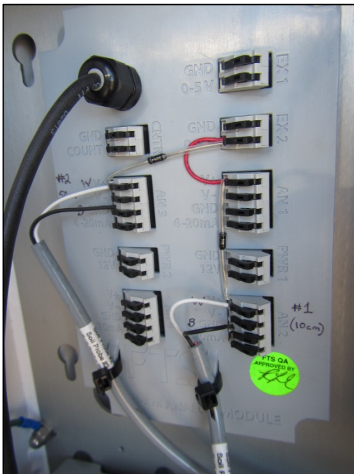
Figure 44. Pfaff Mine RAWs – Wiring configuration used on the replacement analog/digital convertor that accommodates dual soil temperature sensors through SDI.
