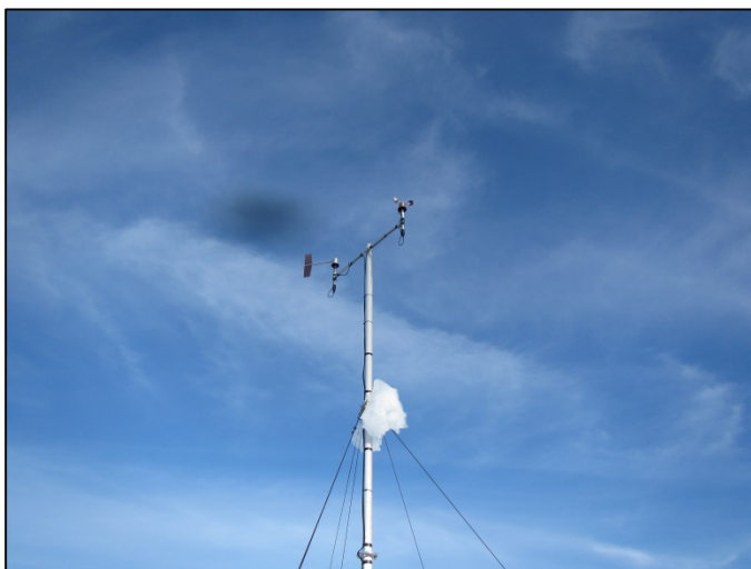
Figure 22. Harding Icefield RAWS – Wind direction sensor without tip.
