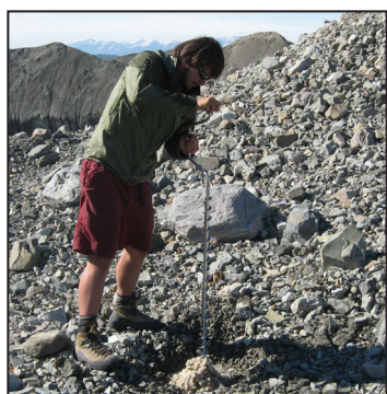
Leif Anderson removed the debris cover at 74 locations on the Kennicott Glacier to drill into the ice. By placing a stake in the drilled hole and replacing the debris, he later could measure the ice melt beneath different thickness of the debris.
