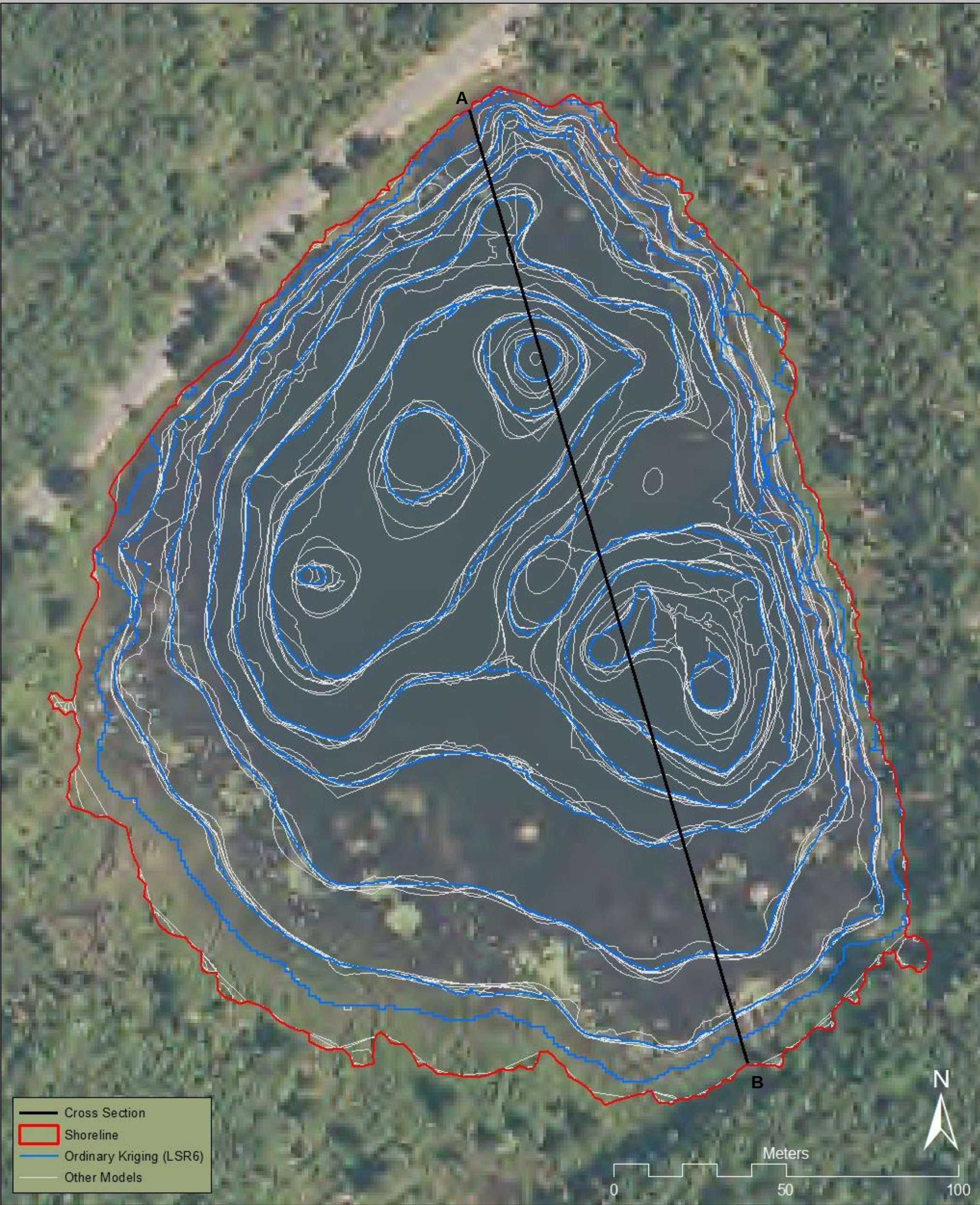
Figure 4. Beaver Dam Pond shoreline and half meter depth contours created from different bathymetric models.
