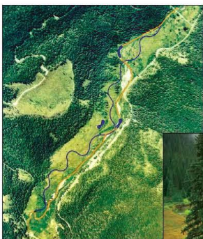
Figure 3. Middle Tepee Creek after reconstruction of meanders and revegetation, 2008.
