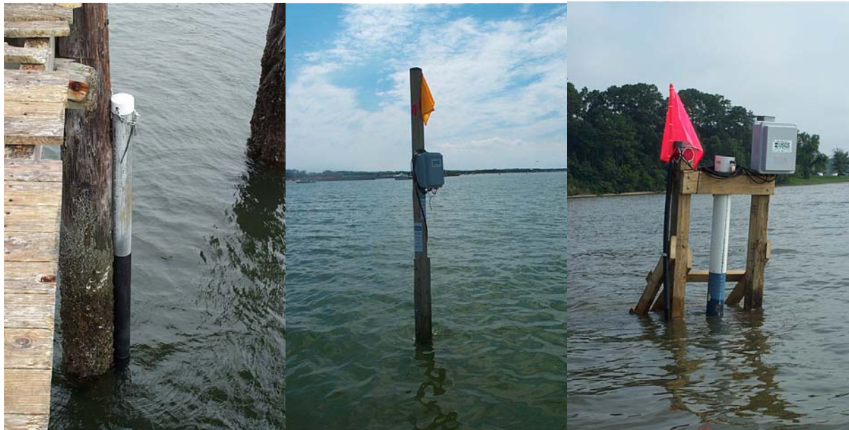
Figure 21. Logging stations for the 2003 feasibility test. (a) at NYPD Pier, Floyd Bennett Field, GATE; (b) temporary 4x4 piling jetted in near Bennett Beach, FIIS; (c) logging platform installed in the style of the VA-Chesapeake NERR at COLO.
