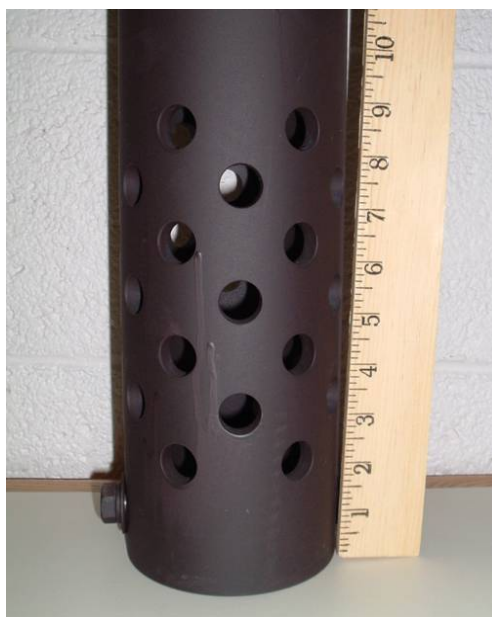
Figure 22. Example of a mounting pipe for YSI 6600-series sondes. The bottom of the pipe is drilled with 0.75" holes on 2.0" centers. A 0.5" bolt is installed through the bottom as a stop for the sonde. Photo courtesy of Mike Lizotte, YSI, Inc.
