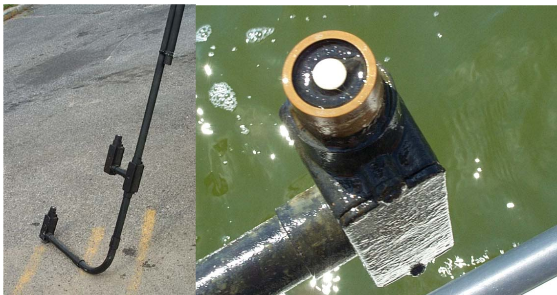
Figure 24. Separate mounting bracket for PAR sensors. The bracket is constructed of PVC conduit and fabricated to hold two upward looking LiCor PAR sensors 50 cm apart (in depth). The upper arm is shorter than the lower arm to prevent shading of the lower PAR sensor. Note that although the bracket is painted with marine non-ablative antifouling paint (Interlux brand ULTRA™ or Petit brand Trinidad SR™), biofouling is still present on the bracket and PAR sensors after four weeks despite weekly trips to clean the sensor (b).
