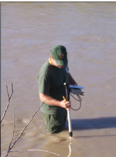
Figure 1. Sampling water velocity on the Arkansas River.
