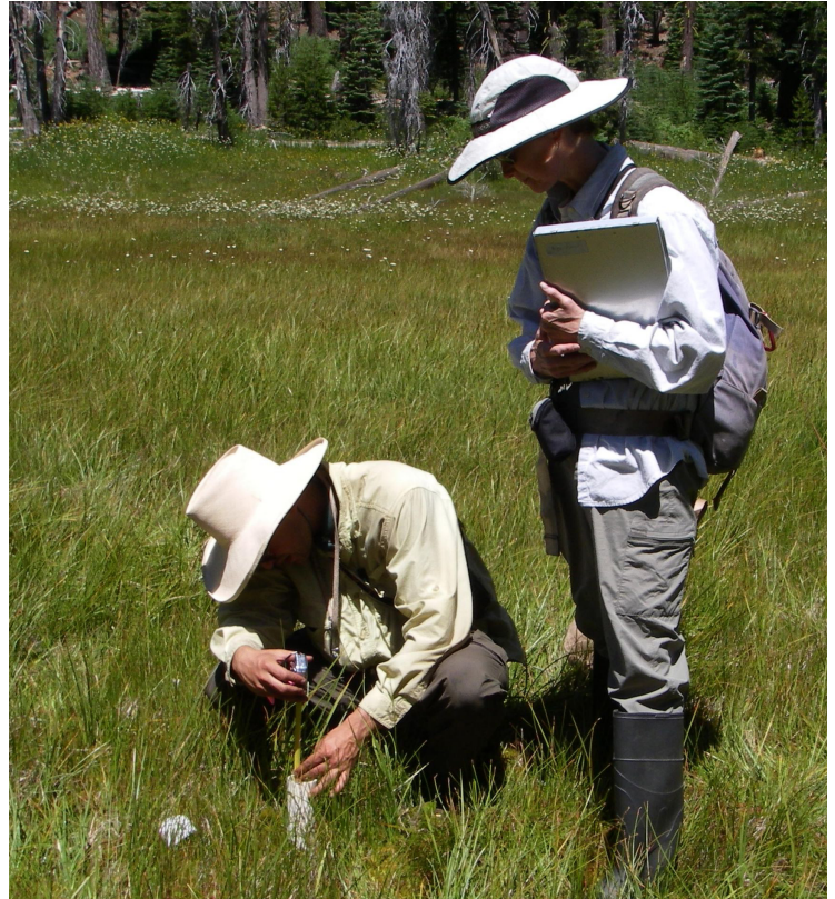
Measuring depth to water level in a groundwater monitoring well, Yosemite National Park. NPS photo.
