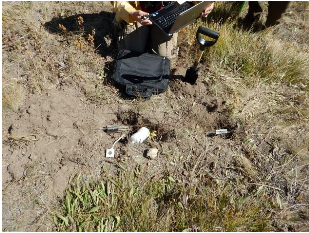
Installing and programming soil sensors
