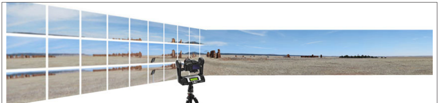
Figure 4. GigaPan uses a robotic camera mount combined with stitching software to join a series of images into a single high-resolution panoramic image.
