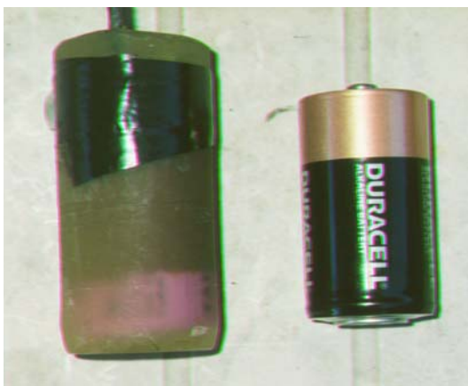
Image 3 Juvenile sized transmitter, shown beside a C- cell battery.
