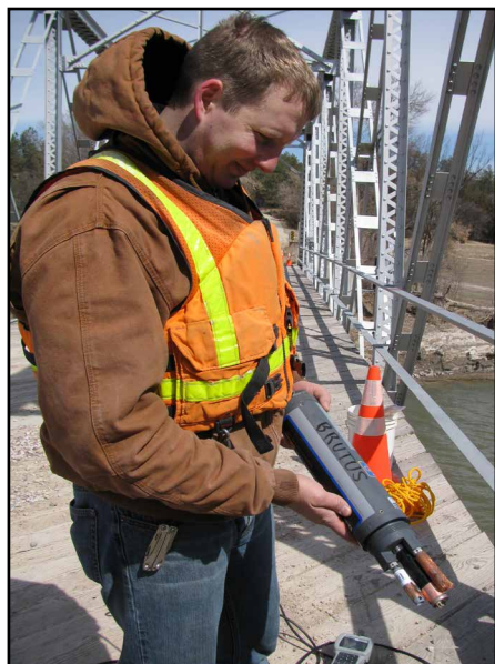
Matt Moser from USGS Nebraska Water Science Center deploying a multi-parameter sonde at Niobrara NSR.
