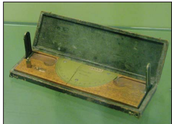
Figure 4: Hand- held inclinometers from Germany were on display in the cartography section in the Deutsches Museum. The one shown was made in Munich around 1860, and with this instrument it would be possible to align the case along a string between stations or use the flip-up alidade sights.
