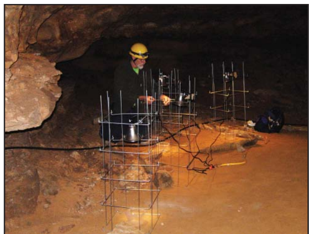
Figure 3. Mammoth Cave ecologist, Rick Olson, sets up an experimental apparatus to measure the amount of algae growth that occurs under different lighting conditions. MCICSL is co-lead on this project, which is also taking place at four other national parks.
