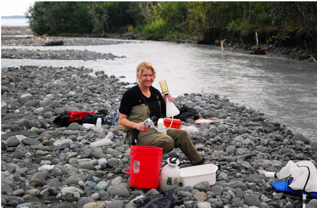
Figure 2. Filtering water chemistry samples in the field (Independence Creek, WRST).
