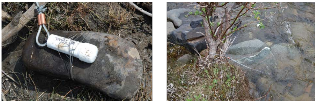
Figure 3. Deployment of temperature dataloggers. The image on the left shows the attachment of the logger to the anchor rock with 20 gauge wire, and to the vinyl-coated steel cable with a cable sleeve and wire clip. The image on the right shows a deployed logger anchored to a riparian tree, which is the preferred method.
