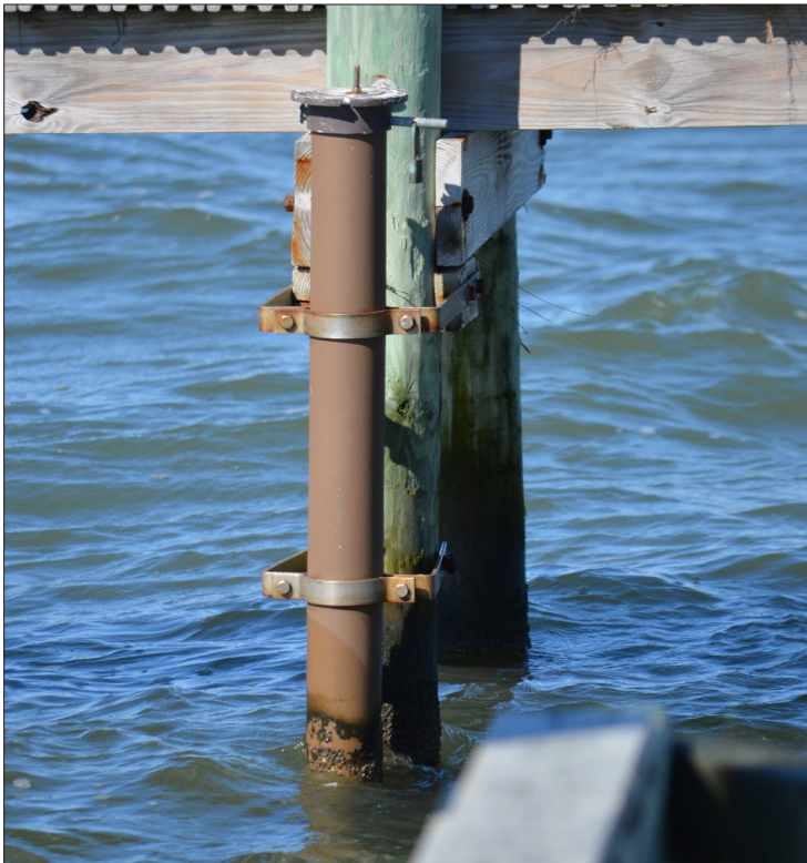
Figure 3. Continuous data collection platform on the Ocracoke boat ramp dock near the Cape Hatteras visitor center parking lot. Photo by Jocelyn Wright, NPS.
