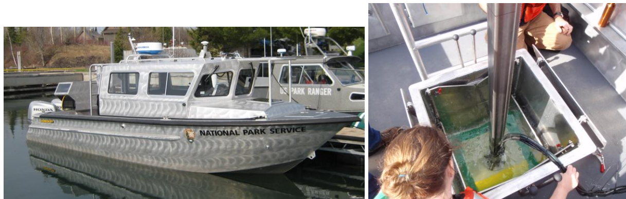
Figure 2. Left: The R/V Echo is a 28-foot vessel equipped with a multibeam sonar system. A generator (seen mounted under a cover on the transom) provides the necessary power to run the sonar system and associated computers. Right: the multibeam sonar head is lowered through a well in the stern deck.
