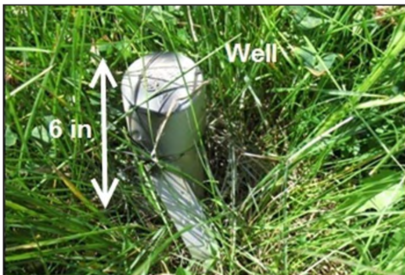
Figure 25. Painted, capped, and tagged groundwater monitoring well in wet meadow. The short elevation of well casings (<6 in.) and high plant productivity typically render wells nearly invisible.
