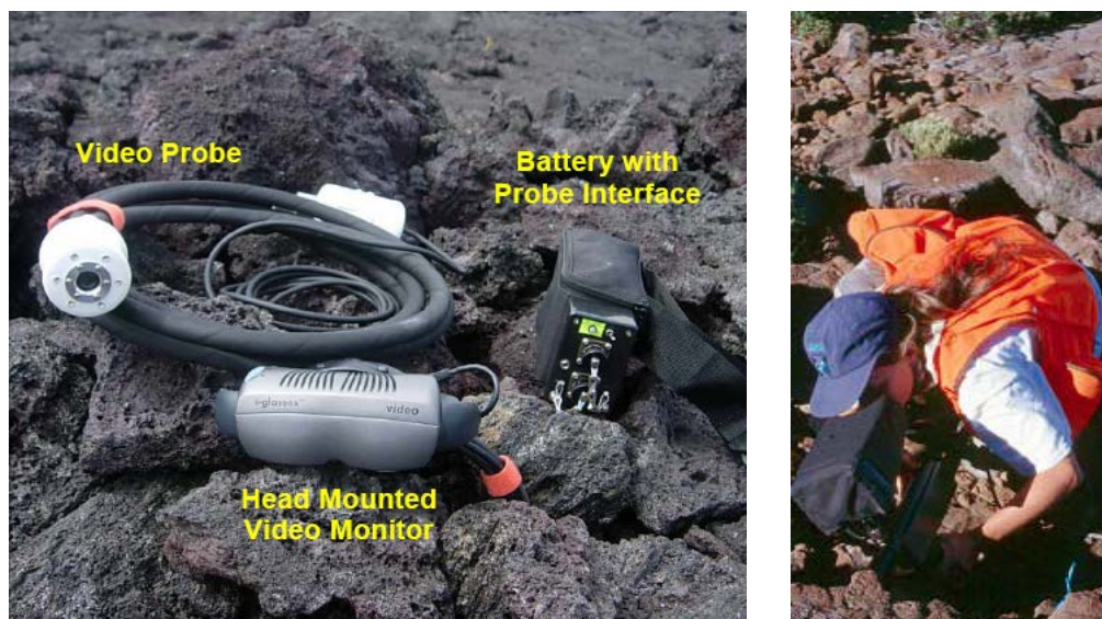
Figure S7.2 (a) Peeper 2000™ burrowscope system, and (b) observer examining a nest chamber with a similar burrowscope system.
