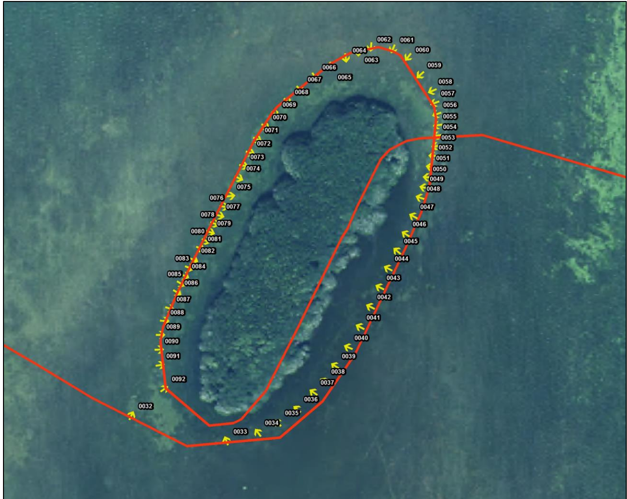
Figure 12. Flight path around Arsenicker Key with photograph locations geotagged. Yellow arrows show direction camera was pointing.
