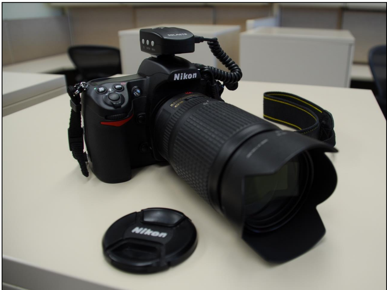
Figure SOP C-1. Shown is the Nikon D300s camera with the vibration-reducing lens and the Solmeta Geotagger attached.
