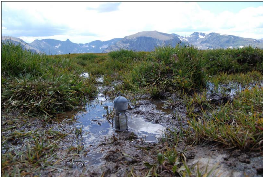
Figure 6-2. Close-up photograph of well casing cut near to the ground and painted to camouflage. Note well armor is not in place on this well.
