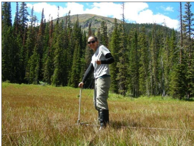
Figure 9-1. Removing water from a well using a bailer.
