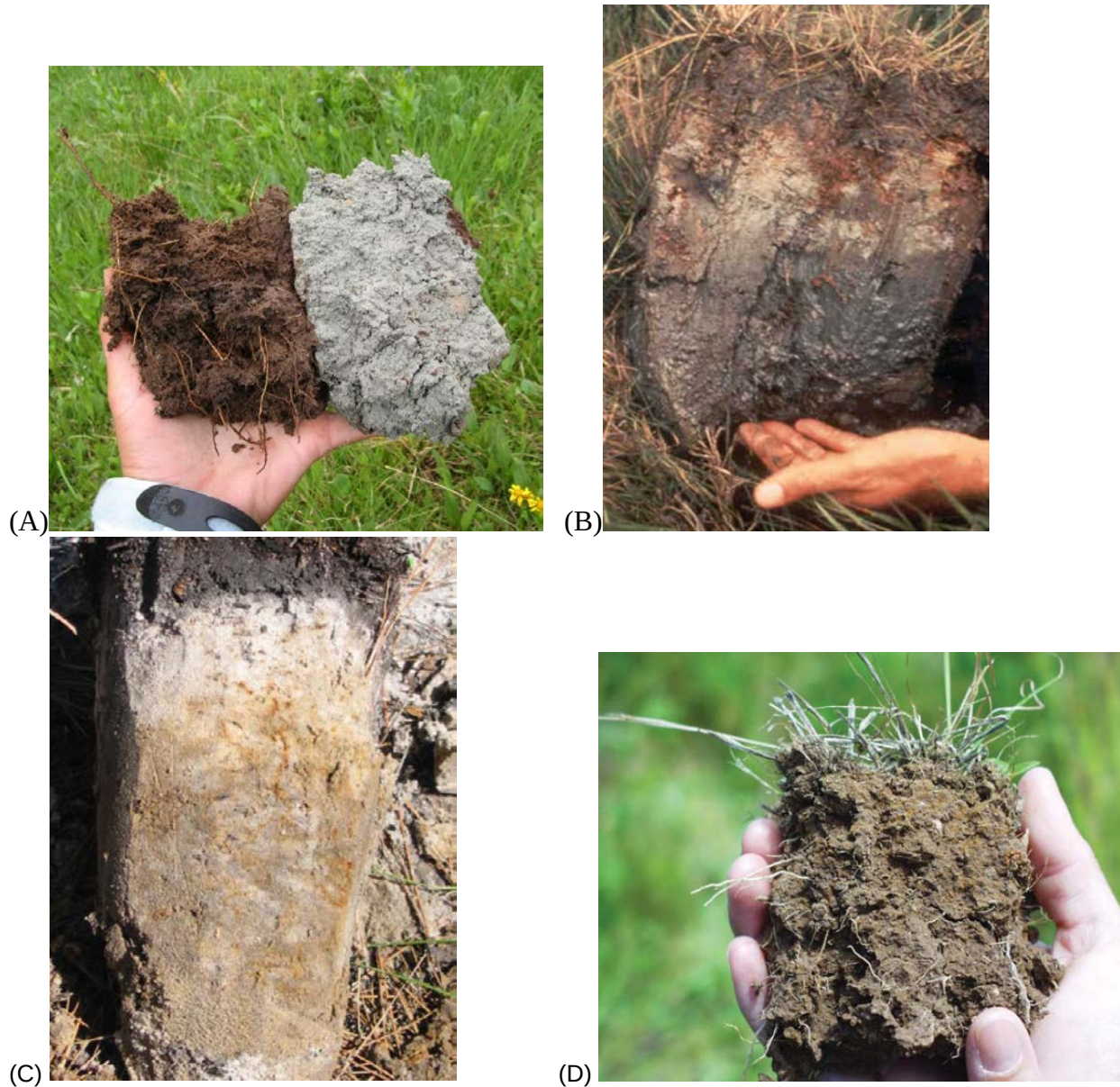
Figure 10-4. Examples of hydric soil indicators: (A) strongly gleyed soil (on the right), (B) loamy gleyed matrix, (C) sandy redox masses removed from hand auger, (D) oxidized root channels visible against matrix color. (Image in A is from B. Schweiger, B-D courtesy of USDA 2006)
