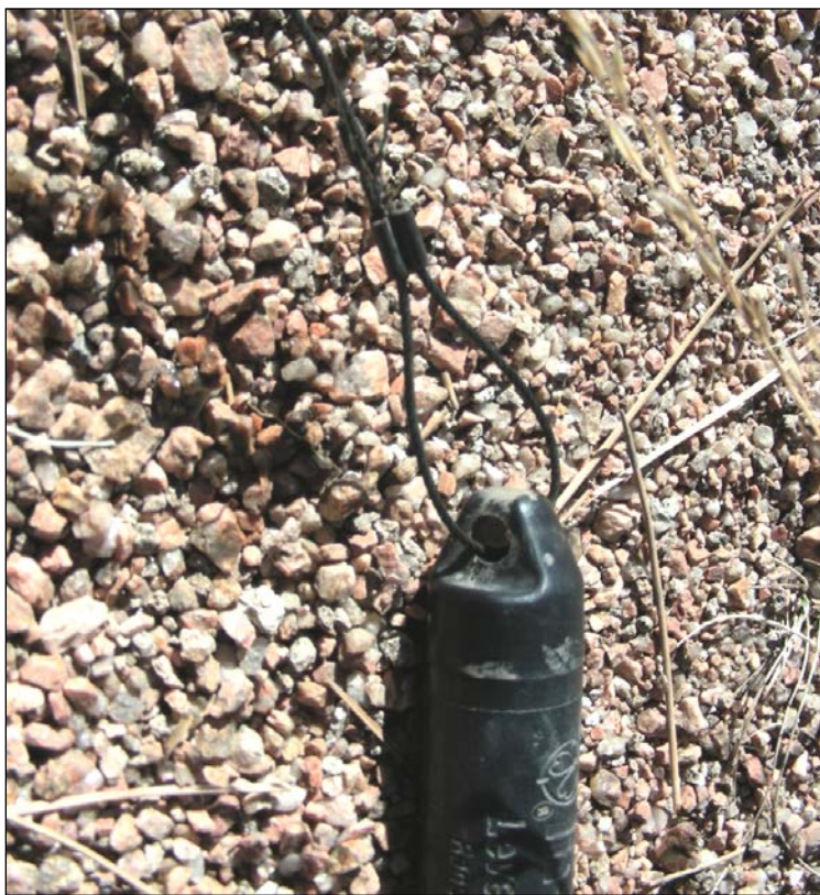
Figure 8-1. Photo of suspension cable used to hang Troll 100/300.
