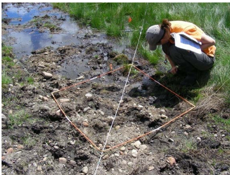
Figure 11-2. Light weight 1x1 m microplot sample frame constructed from wood dowels painted orange and marked in 10 cm increments. The ropes used for the plot as a whole that demarcate the larger plots are also visible. Site is a disturbed wetland in Moraine Park, ROMO.
