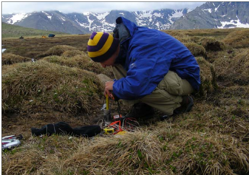
Figure 7-1. Direct manual measurement of water table depths using a volt meter.
