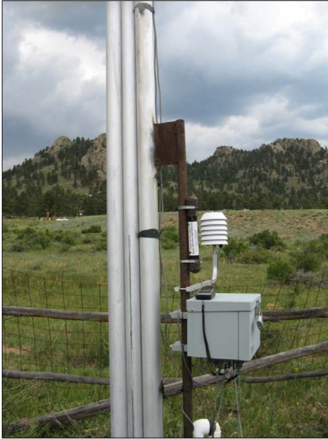
Figure 8-3. Barologger installed on a ROMO weather station.
