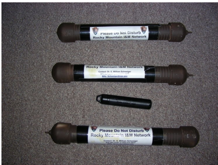
Figure 8-2. Barologger housing with ROMN label. A Troll 100 logger is pictured in between the middle and bottom housings.
